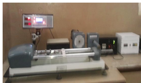
Figure 2 Electronic tensometer used for uniaxial tension test.
