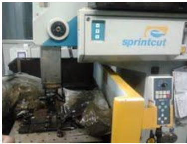
Figure 1 T90Mn2W50Cr45 tool steel material mounted on WEDM.
