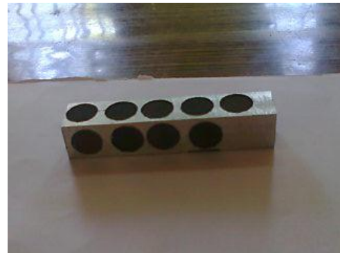
Figure 10 Photograph of machined composite.
