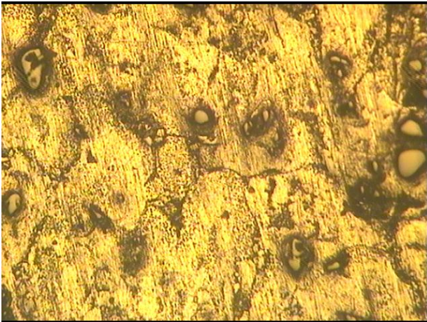
Figure 1 Microstructure of AA6061 wt.5% B 4 Cp composite before machining.
