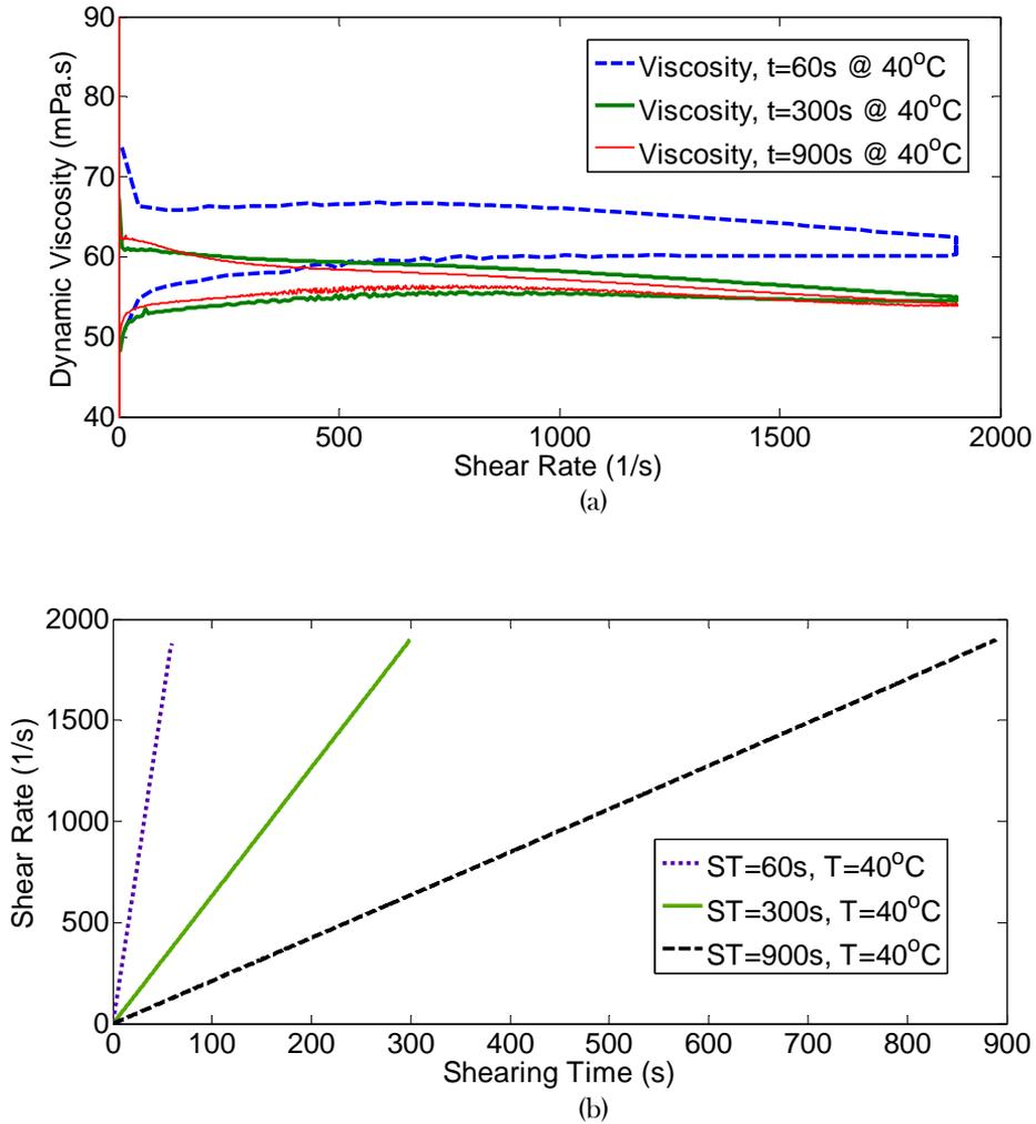
**Figure 2** Viscosity measurements separately at 60, 300 and 900 s shearing time at 40 degree Celsius. Graph (a) represents viscosity versus shear rate, and graph (b) represents shear rate versus shearing time
