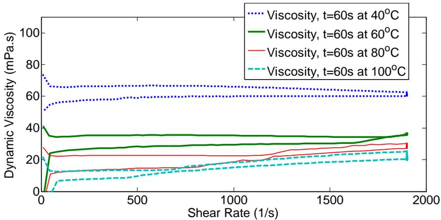
**Figure 4** Viscosity versus shear rate at 60 s shearing time at respective 40, 60, 80 and 100 degree Celsius
