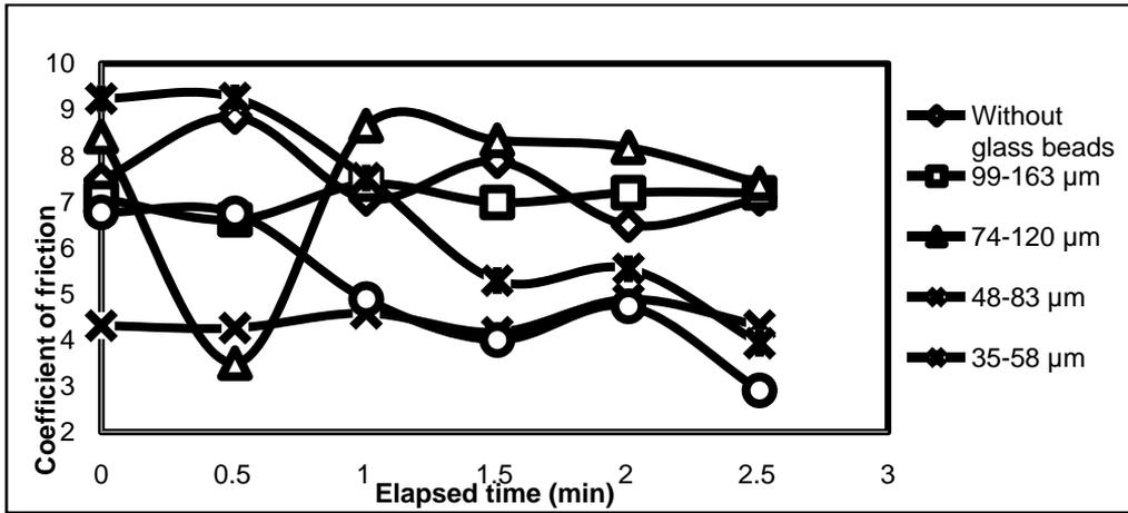
Figure 7 Coefficient of friction vs elapsed time
