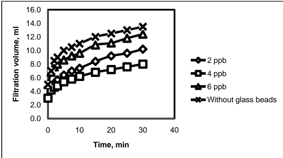
**Figure 6** Filtration volume for different 48-83  $\mu\text{m}$  glass bead concentrations
