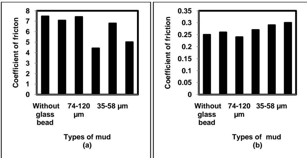
Figure 8 Average coefficient of friction value using (a) LEM-4100, and (b) Fann lubricity tester
