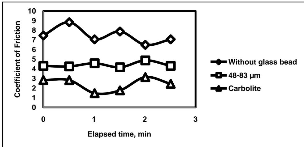
**Figure 9** Comparison the coefficient of friction between glass beads and carbolite
