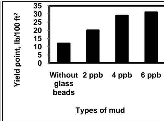
**Figure 4** Yield point for different 48-83  $\mu\text{m}$  glass bead concentrations
