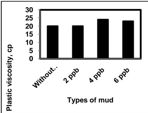
**Figure 3** Plastic viscosity for different 48-83  $\mu\text{m}$  glass bead concentrations
