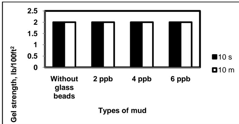
**Figure 5** Gel strength for different 48-83  $\mu\text{m}$  glass bead concentrations
