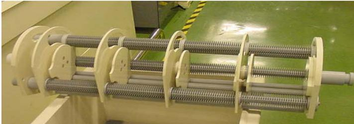
**Figure 4** New etching drum
