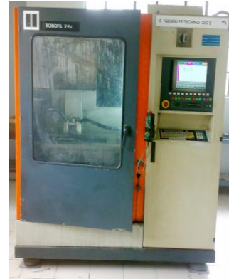
Figure 3 Wire EDM Robofil-290 (Courtesy by Charmilles Technologies)
