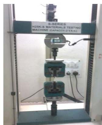
Figure 1 Specimen placed in UTM
