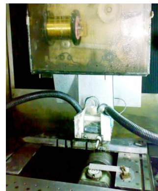
Figure 4 WEDM of workpiece
