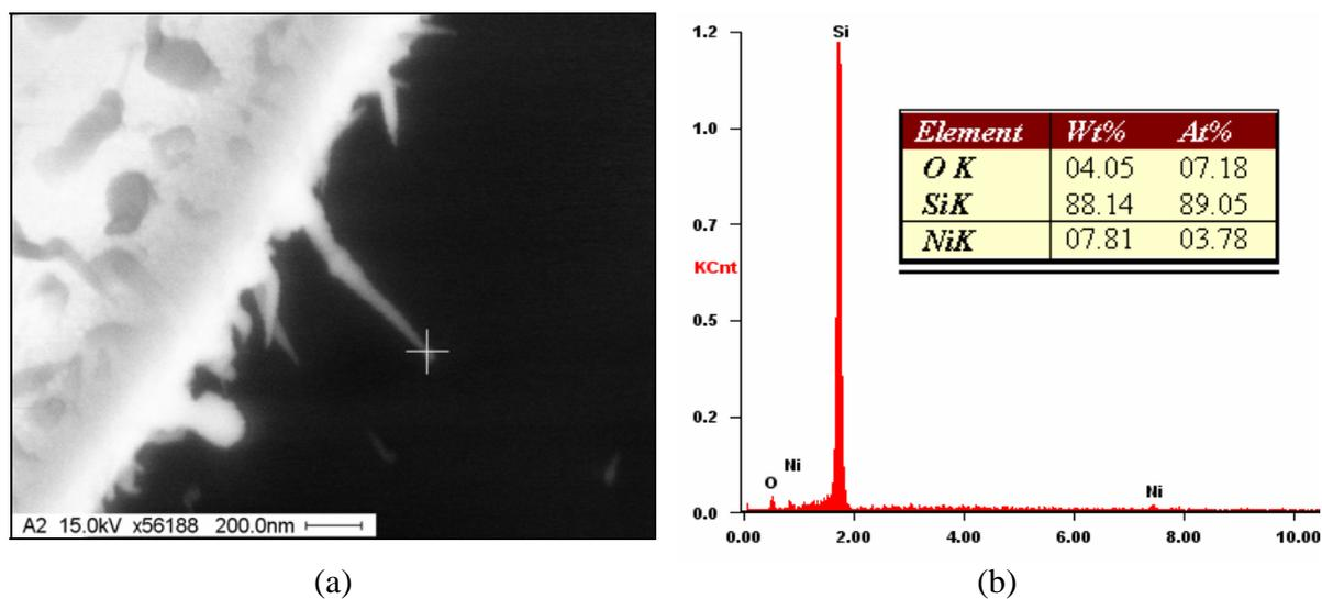
Figure 3: (a) FESEM image shows one dimensional nanostructure with sphere at the tip, (b) EDX analysis recorded elemental composition of the tip: 89.05 at% Si, 7.18 at% O and 3.78 at% Ni.
