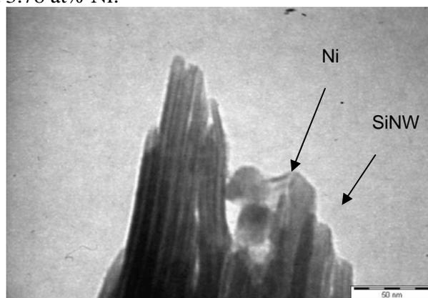
Figure 4: TEM image shows silicon nanowhisker with nanosphere at the tip.
