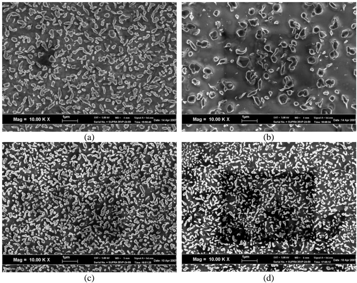
Figure 2: FESEM images of Si nanostructures obtained at substrate location (a) 3 cm, (b) 6 cm, (c) 9 cm, and (d) 12 cm away from source material.
