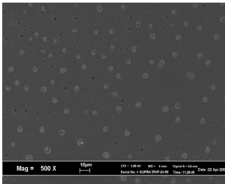
Figure 1: FESEM image of nickel-coated Si substrate.
