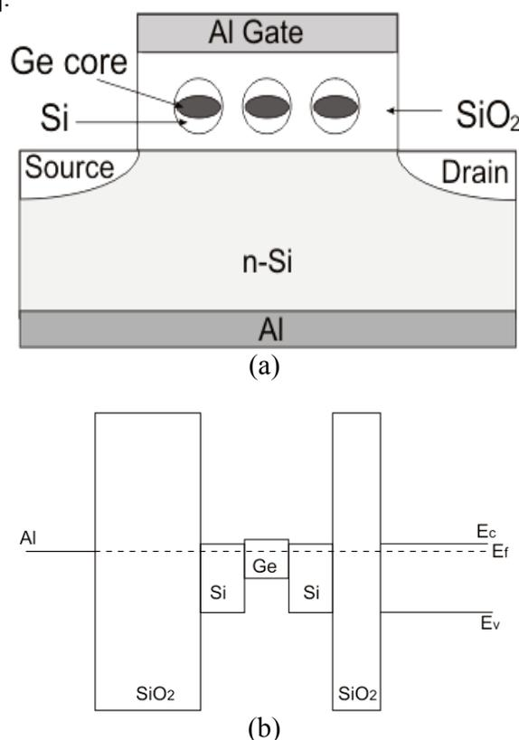
Figure 1: Schematic diagram of the memory device using Si dot with Ge core as floating gates (a) accompanied with their energy band structure (b).
