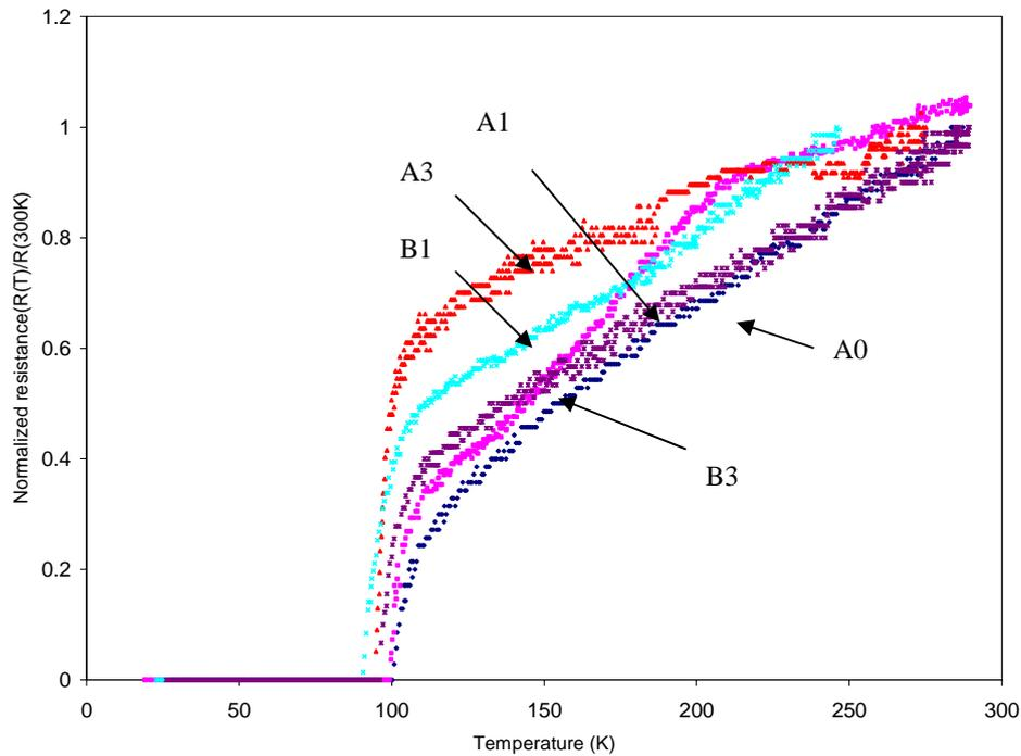
Figure 3: The variation of resistivity with temperature for  $Tl_2Ba_2CaCu_2O_{8-(Ag_3)_x}$  with  $x = 0$  and 1 wt% and 3 wt%.
