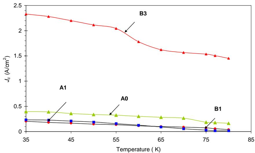
Figure 4: Temperature dependence of  $J_c$  in  $Tl_2Ba_2CaCu_2O_{8-(Ag_3)_x}$  for  $x = 0-3$ wt%.
