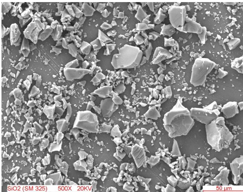
Figure 1: Scanning electron micrograph of the silica powder showing the fracture particles with irregular edges and surface
