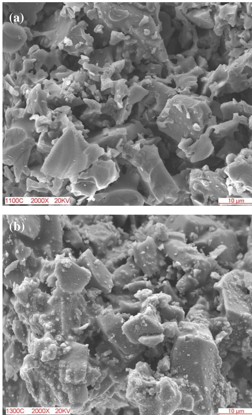
Figure 3: Scanning electron micrograph of the sintered silica F2 body at 1100°C (a) and 1300°C (b) showing the arrangement of the particles and the pores in the body.
