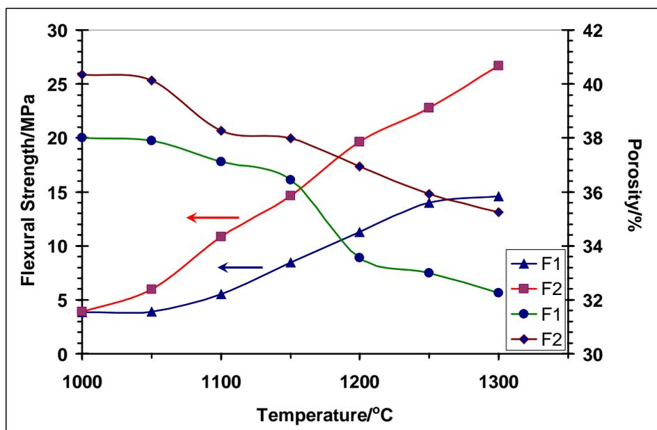
Figure 4: The porosity and flexural strength of the filter samples versus the respective sintering temperatures.
