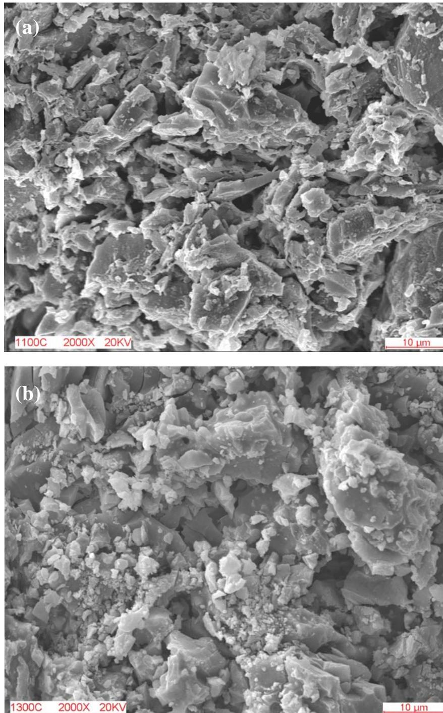
Figure 2: Scanning electron micrograph of the sintered silica F1 body at 1100°C (a) and 1300°C (b) showing the arrangement of the particles and the pores in the body.
