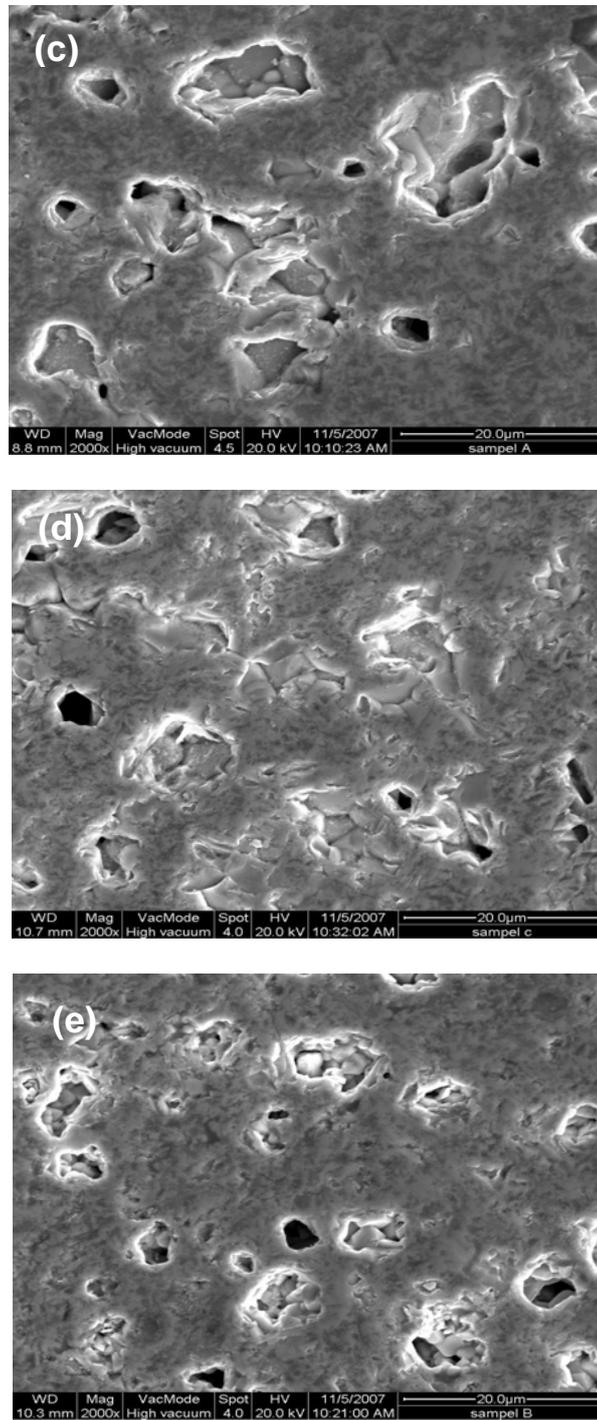
Figure1: SEM micrographs of doped concentration of Pr (a) X1(x=0); (b) X2(x=0.1); (c) X3( x=0.2); (d) X4(x=0.3) and (e) X5(x=0.4).
