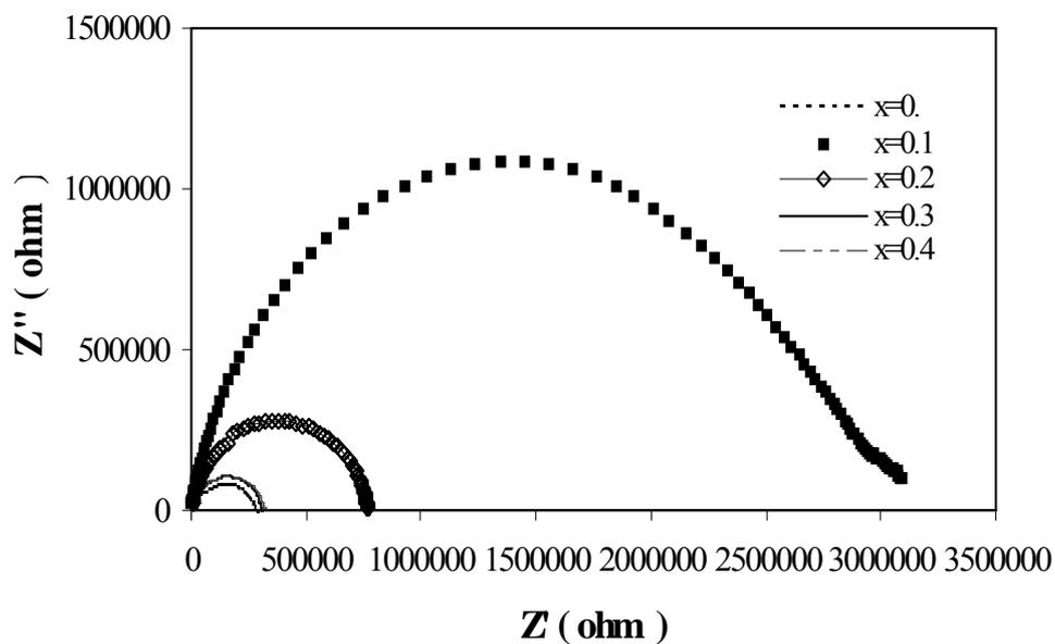
Figure 5: Complex impedance Nyquist plot at different x concentration.
