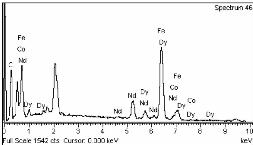
Figure 3(b): Quantitative analysis of compacted bonded magnet.
