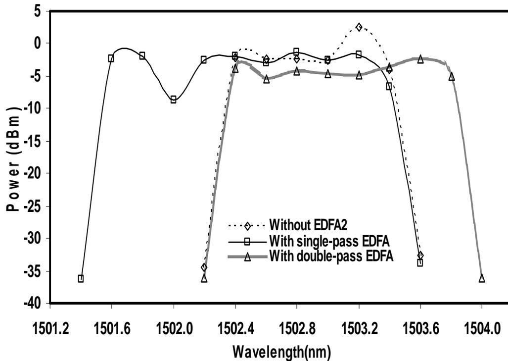
Figure 3: Tuning characteristics for different BEFL schemes.
