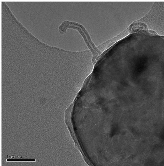
Figure 5: TEM micrograph of individual CNTs
