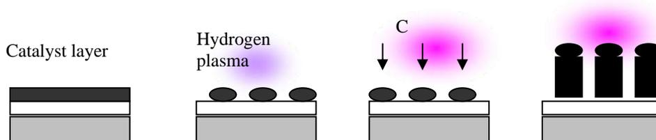
Figure 2: Schematic of growth mechanisms of CNTs
