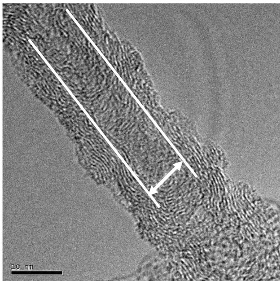
Figure 6: TEM micrograph of multiwalled CNTs
