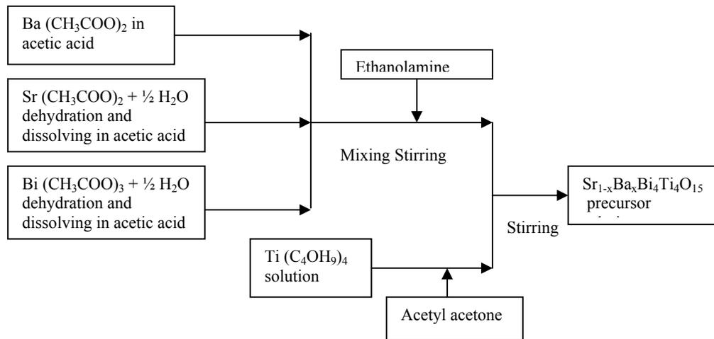
Figure 1: Flow chart of the fabrication process of SBBT.
