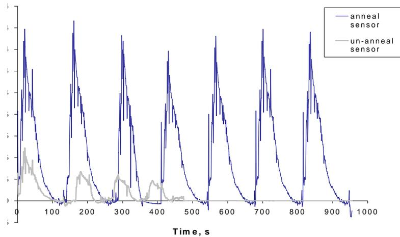
Figure 7: Voltage response of the SBBT thin films pressure sensor measures at pressure 450 kPa for seven cycles.
