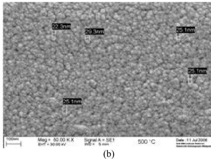
Figure 4: SEM photo of surface morphology of SBBT thin film (a) un-anneal and (b) anneal at 500°C temperature
