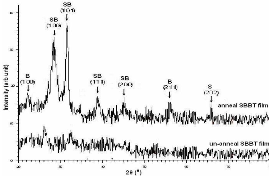
Figure 6: XRD patterns of  $\text{Sr}_{0.5}\text{Ba}_{0.5}\text{Bi}_4\text{Ti}_4\text{O}_{15}$  thin films for un-annealed and annealed at 500°C ( S denotes  $\text{SrBi}_4\text{Ti}_4\text{O}_{15}$  phase and B denotes  $\text{BaBi}_4\text{Ti}_4\text{O}_{15}$  phase).
