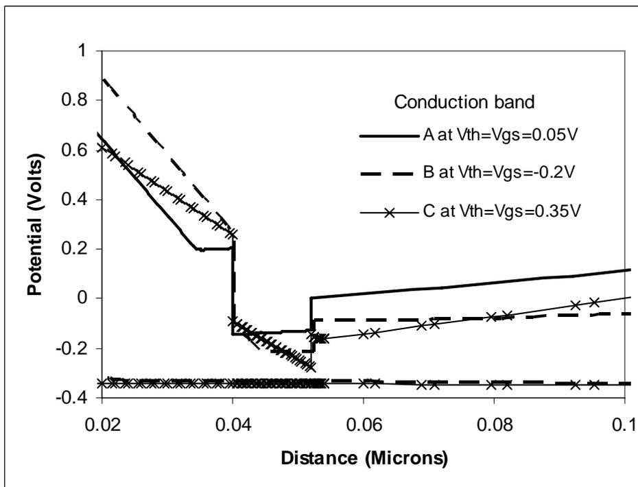
Figure 4(a): Conduction band at 0V biased
